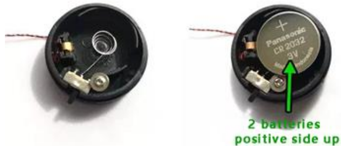
Button battery box (round) battery correct installation
