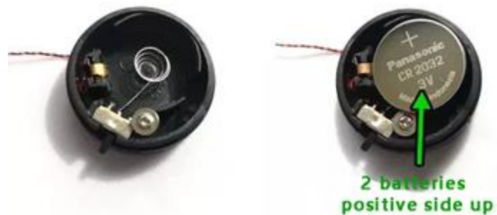
Button battery box (round) battery correct installation
