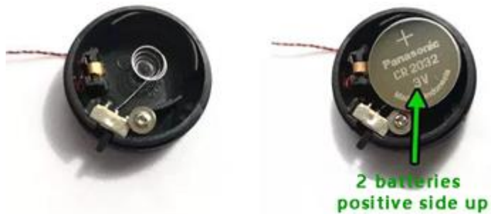
Button battery box (round) battery correct installation
