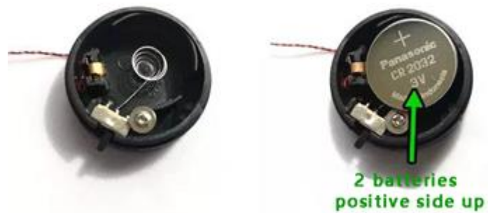
Button battery box (round) battery correct installation
