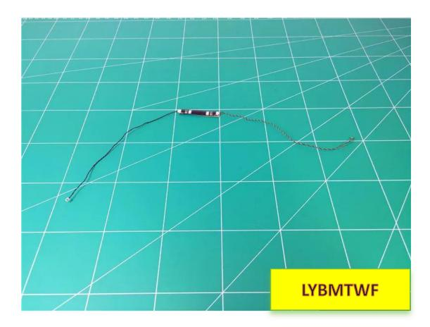
Take out the 4-seater socket and USB cable, connect them to the light group, connect the power supply, and test whether the light particles light up normally.
