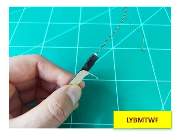
Attach the light strip to the position shown in the figure. Note that the light wire is on top . Remove the black L-shaped part indicated by the arrow.
