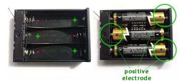
Button battery box (flat) battery correct installation method
