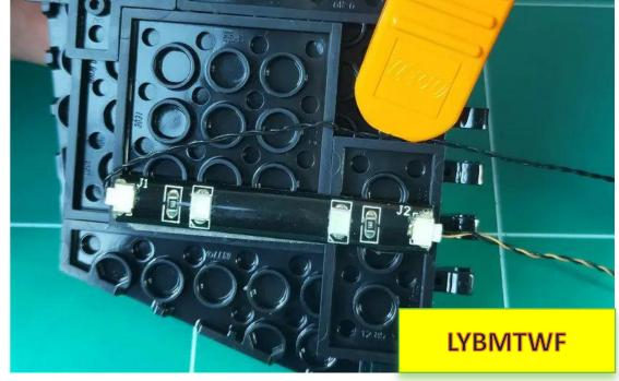
Restore the black L-shaped parts and fix the connecting wires
