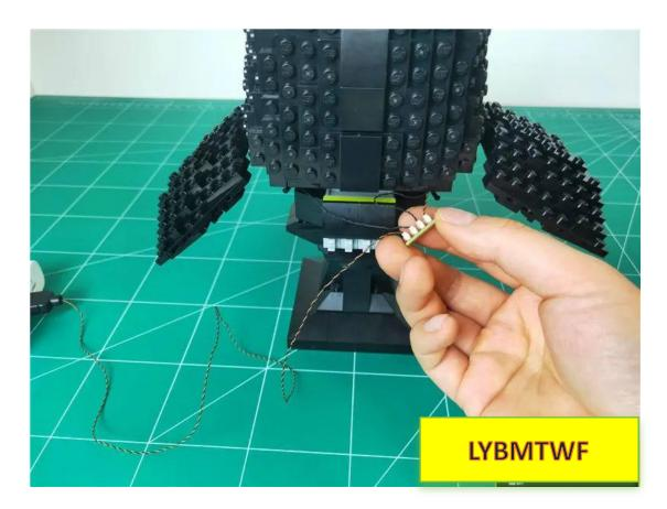
Take out the 4 sockets connected to the USB cable and insert all the wires into the 4 sockets
