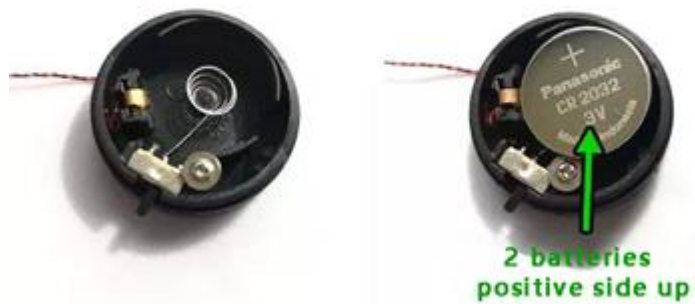
Button battery box (round) battery correct installation
