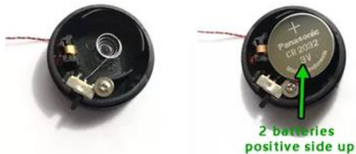
Button battery box (round) battery correct installation
