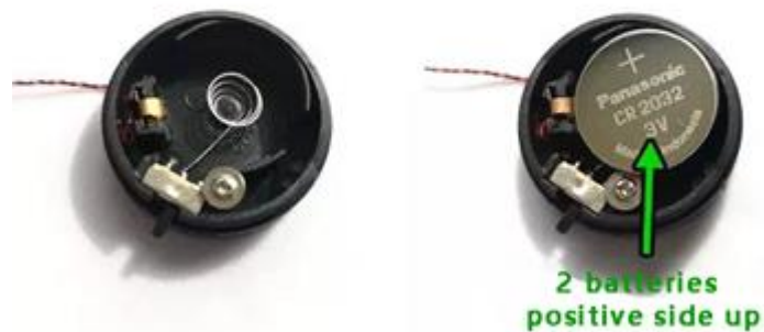
Button battery box (round) battery correct installation
