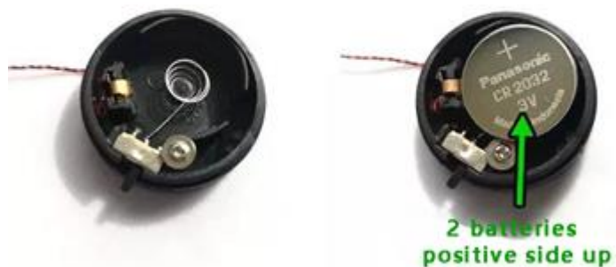
Button battery box (round) battery correct installation
