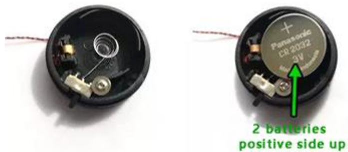
Button battery box (round) battery correct installation
