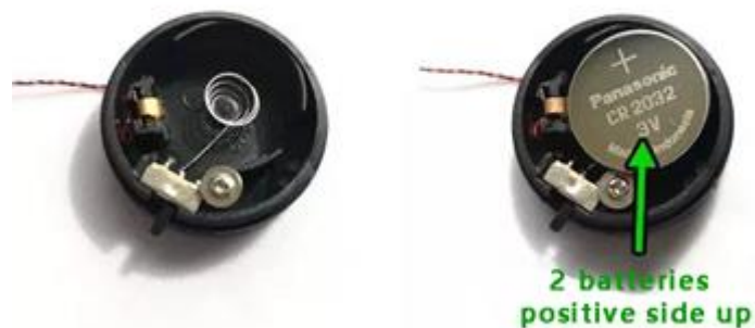
Button battery box (round) battery correct installation
