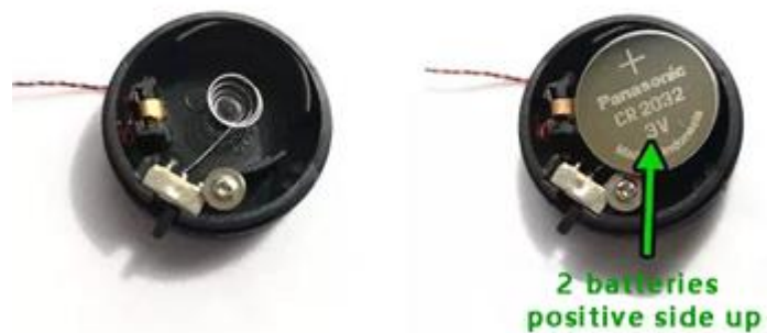
Button battery box (round) battery correct installation
