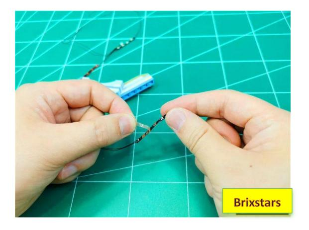
Paste the light strip to the edge of the blue part shown in the figure, leaving two light points at the top empty.
