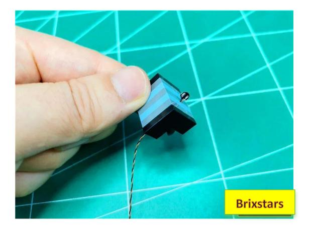
Attach the light pellets to the roof with the light-emitting side facing upwards
