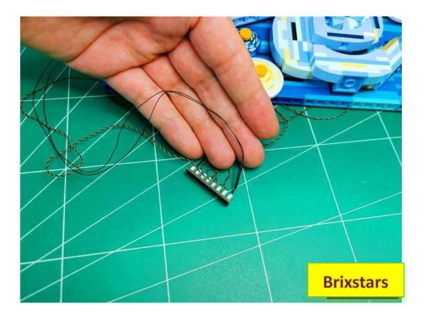
Turn on the power, test that the light is on normally, and turn off the power after the test is completed.
