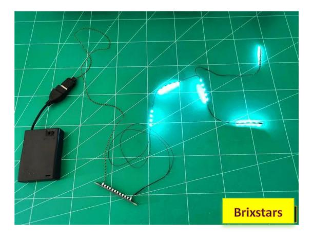
After the test, turn off the power, unplug the light strip, and leave the socket on the power supply
