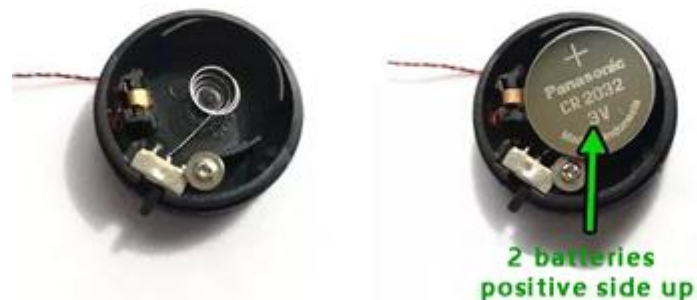
Button battery box (round) battery correct installation
