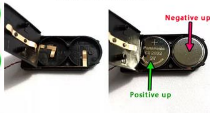
Button battery box (flat) battery correct installation method
