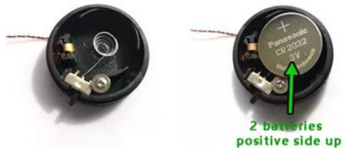
Button battery box (round) battery correct installation
