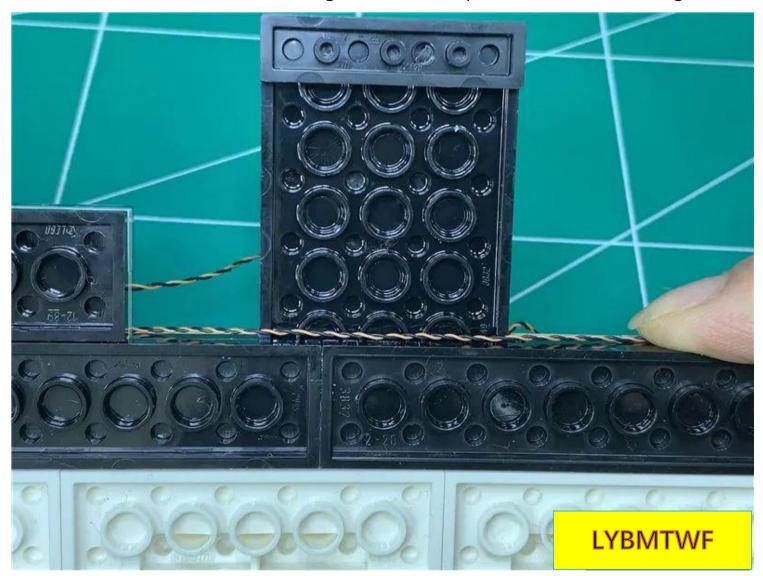
Fit the wire at the corner to the edge of the black part, as shown in the figure
