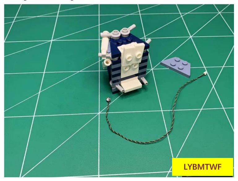
Attach the lamp to the white part, with the light-emitting surface facing u pward and the wire facing right, as shown in the figure.
