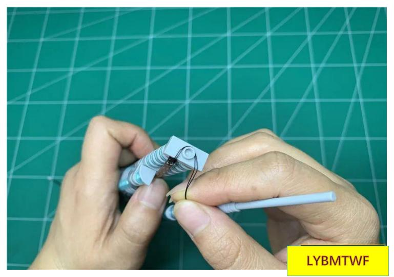
Restore the spire and fix the wires. Note that the spire wires and the light strip are on the same side.
