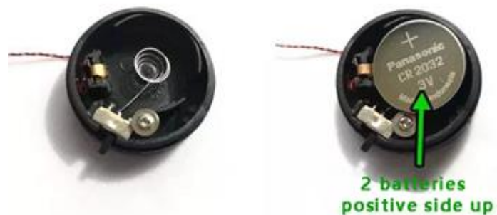
Button battery box (round) battery correct installation
