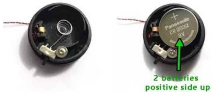
Button battery box (round) battery correct installation
