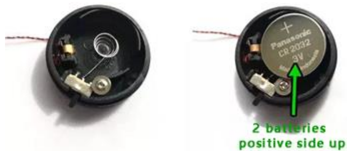
Button battery box (round) battery correct installation
