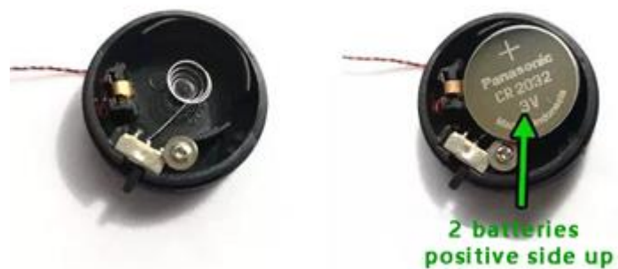
Button battery box (round) battery correct installation
