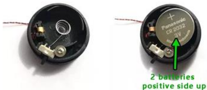
Button battery box (round) battery correct installation
