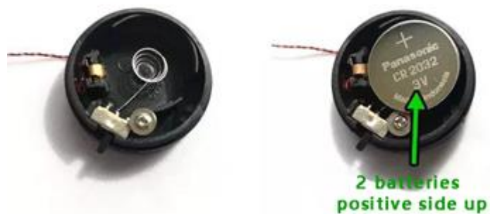
Button battery box (round) battery correct installation
