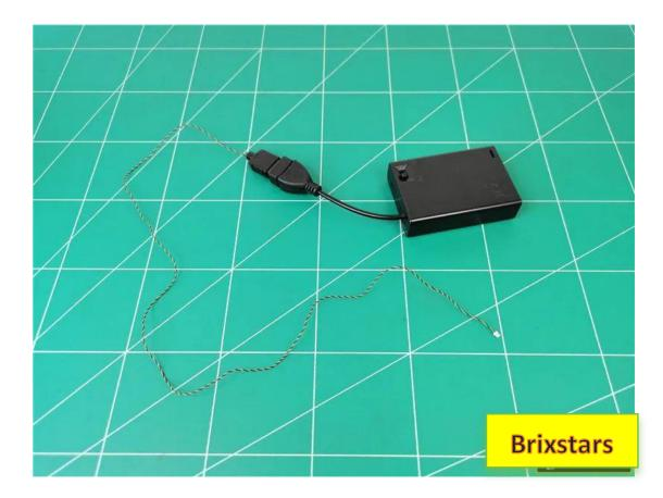
Remove the USB power cable and insert it into the battery box
