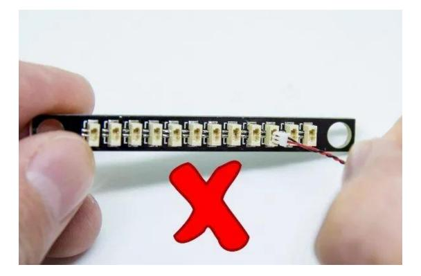
When installing the light pellets on the building blocks, make sure they are properly positioned (with the yellow LED assembly exposed). You can place them directly on top of the building block studs or in between.
