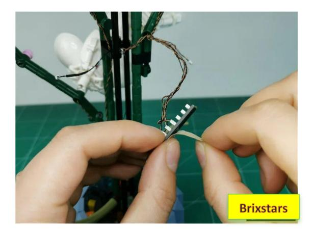
Wrap the wires around the 8-block appropriately and insert the 2 shorter wires into the 8-block
