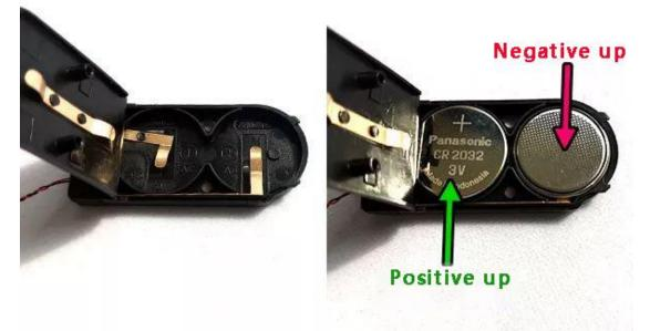
Button battery box (round) battery correct installation
