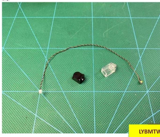
Place the light pellet with the luminous side facing upwards on the black protrusion, **making sure** the wire is facing the concave side of the black part.
