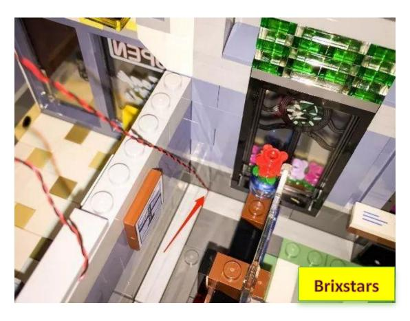
4.) Take out a 6-port socket and connect the lamp post wire to the 1st port of the 6-port socket.
