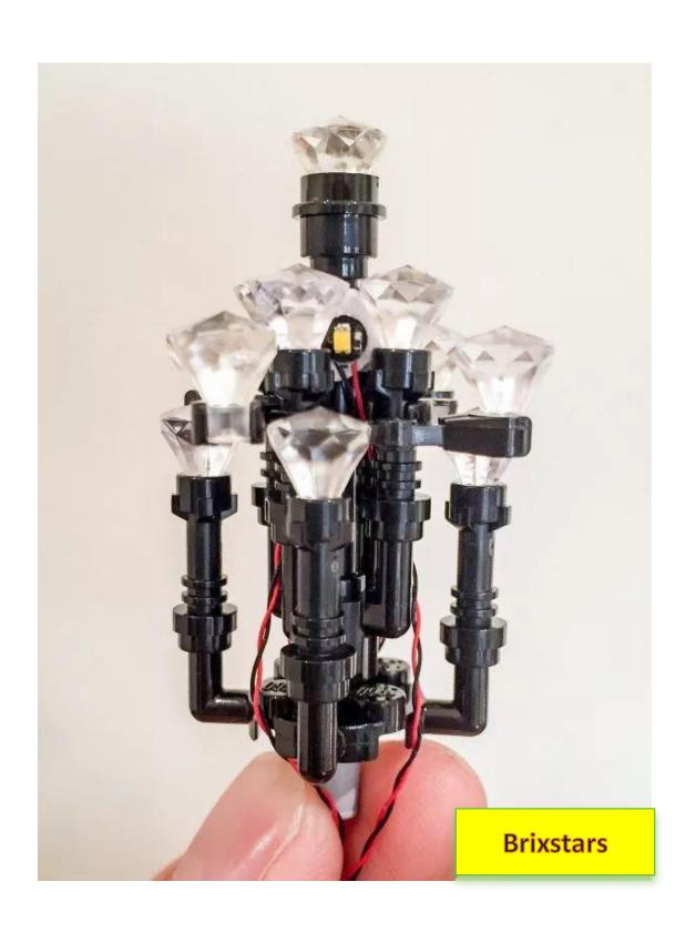
34.) Reassemble the chandelier. As shown in the picture below, connect the 4 lamp wires together and fix them under the white Lego plate.
