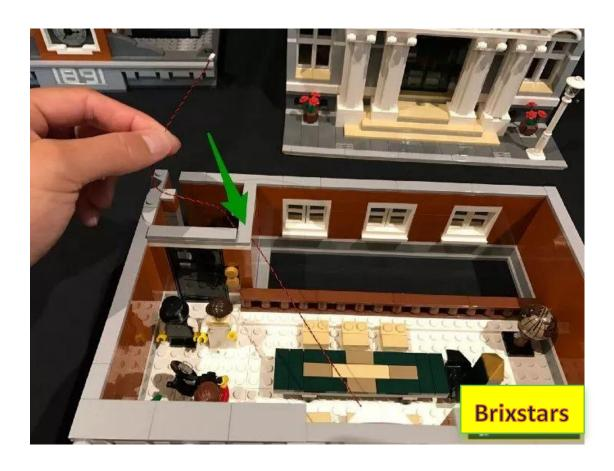
26.) Flip the three layers over and install the other 2 LED strips (strip #4 and strip #5) to the following positions. Use another 15CM connecting wire to connect them together, then take another 15CM connecting wire and connect it to the left port of strip #4 ( to prevent the 15CM wire from hanging down, you can wrap the wire under the strip )
